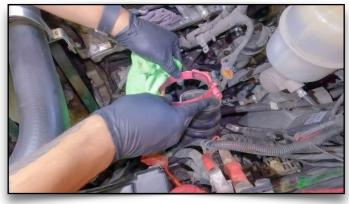
100. Remove Rag From Boost Tube, Put Clamp Back On
