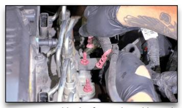
49. Remove Cable Ties from Driver Side Studs
