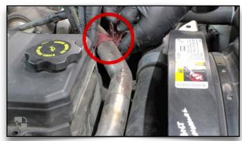
14. Remove and Dispose EGR Tube P-Clamp
