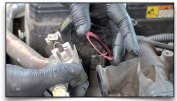
**23. Release Clamp and Remove Gasket**Catch the gasket and put it aside for later, this will be reused.
