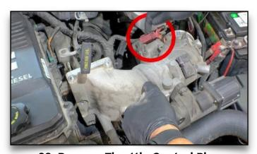
**38. Remove Throttle Control Plug**Now that the elbow has been leaned forward, you can easily reach this plug.
