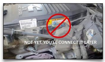
99. Do Not Connect Front Blue Injector Plug Yet
