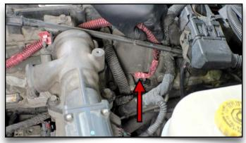
**29. Remove Heater cable from Terminal** Relocate the wire out of the way once the free.
