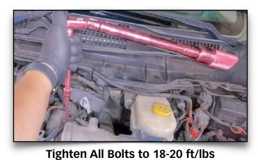
Start with the bolt that's inside the Monster-Ram, then work in a cross pattern to torque to spec.
