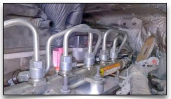
**88. Connect Temp Sensor Extension Harness** Be sure to lock the plug once connected.
