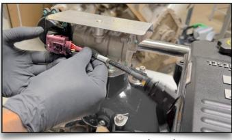
**18. Remove EGR Valve Plug**Press the locking tab, press the plug forward to release tension, then pull back to remove.
