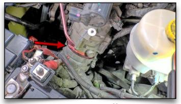
33. Pry Boost Tube Hose Off Throttle Body
