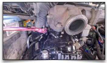
105. Tighten Coil Heater By Hand
