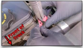
112. Remove & Discard 12V Heater Cable P-Clamp
