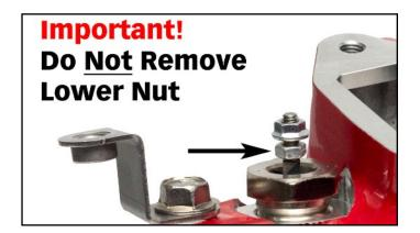
If installing with the Banks High-Flow heater and Billet Plate, the lower locking nut must not be removed from the heater coil. Take care when installing OEM heater wire ring terminal, it must be sandwiched between lower and upper nut.
