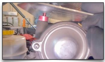
**126. Place Rear Heatshield Spacer & Screw** Use a drop of thread locker on the screw to prevent it from vibrating out.
