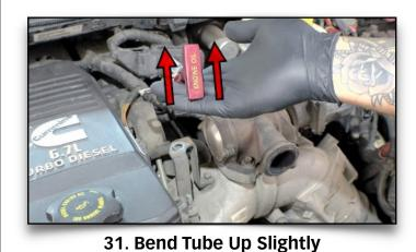
The Monster-Ram is slightly taller than the factory Intake Elbow; you'll fine-tune this bend after the Monster-Ram is installed.
