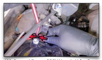
**108. Connect Forward PCV Hose to Valve Cover** This is a tight fit, but doable. Wiggle the rubber hose on the nipple a quarter inch, then use a pry tool as a lever to help slide it on.
