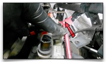
Once the cap is removed, press the small red locking tab in, then unplug the sensor.
