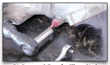
71. Remove & Transfer Elbow Stud
