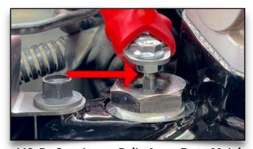
118. Be Sure Lower Bolts Away Form Metal No part of the 12V cable can touch the body of the coil heater. Otherwise it will arc, melt, and fail.
