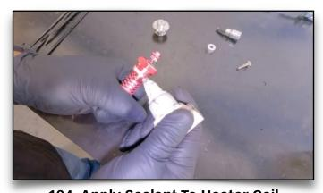
**104. Apply Sealant To Heater Coil** Start with the bolt that's inside the Monster-Ram, then work in a cross pattern to torque to spec.
