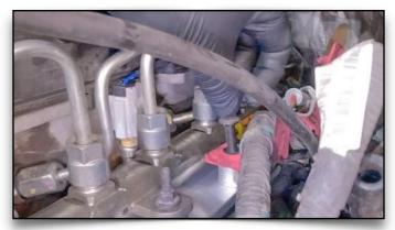
**Slide Dipstick Bracket Over & Reinstall Stud**
