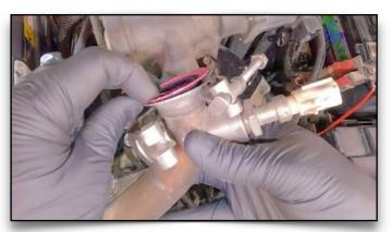
121. Conical Gasket Goes On Driver Side of EGR Tube
