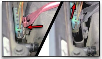
43a. Press in the clip with a flat tool, & pull up.
