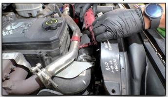
13. Remove Bolt Under Center of EGR Crossover Tube
