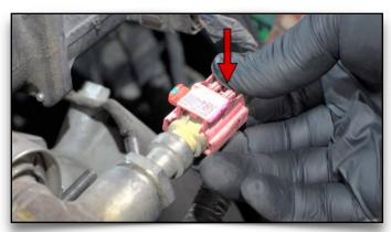
**17. Remove Temp Sensor by Pinching It** Unclip this wire clip for extra clearance.
