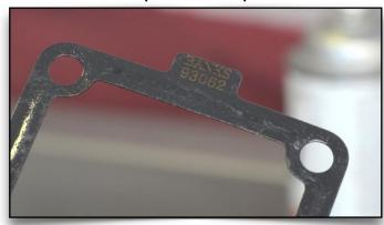
Side that says Banks, should be the side with the adhesive. Let it sit for about 3 min for the glue to tack up.
