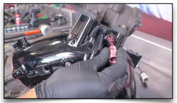
78. Install Rear Thermocouple Plug
