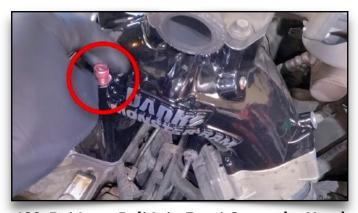
**102. Put Long Bolt Into Front Corner by Hand** This will help hold the Monster-Ram in place. Then do the same for the long bolt on the backside. Followed by the two smaller bolts.
