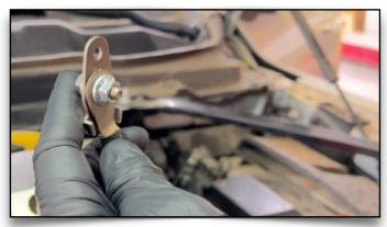
114. Assemble Heater Cable Extension Bracket
