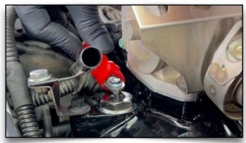
**116. Place Heater Cable Onto Threaded Post** The head of the M6 Bolt you just covered needs to face down.
