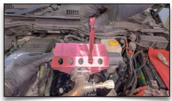
125. Install EGR Heat Shield & Tighten Bolts
