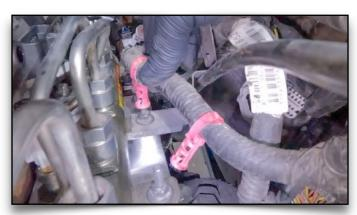
90. Push Engine Harness Cable Ties Back Onto Studs
