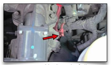
34. Remove Cable Tie Back of Elbow & Unplug MAP sensor
