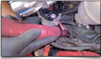
111. Tighten Boost Tubes Clamp
