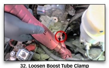
This does not have to be fully removed, just release tension on the hose
