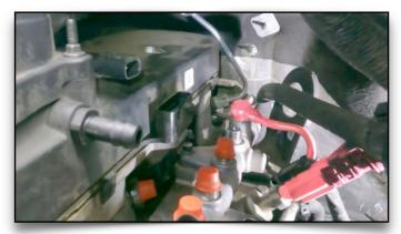
85. Re-Install Temp Sensor. Hand Tighten Washer & Banjo Bolt
