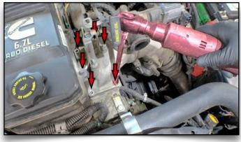
36. Remove 6 Bolts on Elbow
